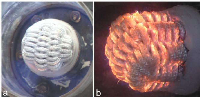
**Figure 1: An experimental braided burner in operation: a) at fuel-lean condition; b) at nearly stoichiometric condition.**
