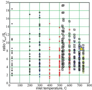
**Figure 6: Ratio of mixture surface speed to laminar burning velocity versus inlet temperature. Experimental conditions are given in Figure 3. Relation to micro turbine operating points: ★ - base load; ◆ - 50% load.**
