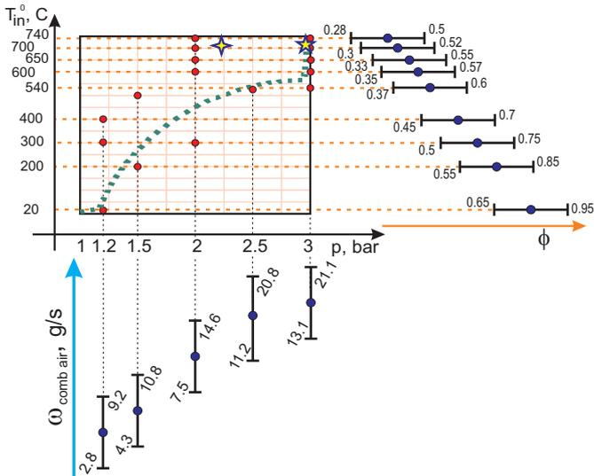
**Figure 3: Experimental points (red circles) and conditions: inlet temperature, pressure, mass flow and equivalence ratio. Relation to micro turbine operating points: ★ - base load; ✦ - 50% load; - - - ramp-up.**
