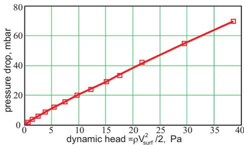
**Figure 4: Non-reacting flow pressure drop over the burner surface versus dynamic head at  $T_{in}=20$  C.**
