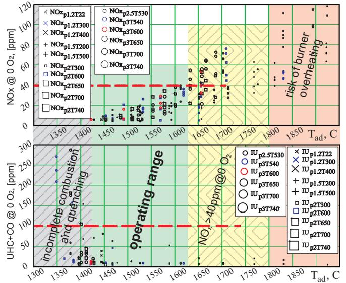
**Figure 7: NO<sub>x</sub> and combined (CO+UHC) mole fractions versus adiabatic flame temperature.  $T_{in}$  and  $p$  are given in the legends: p1-p3 – 1-3 bar; and T22-T740 – 22-740 C. Relation between  $\omega$ ,  $p$ ,  $T_{in}$  and  $\phi$  is given in Figure 3.**
