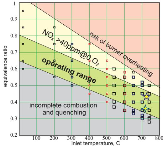
**Figure 9: Experimental points on the plane of equivalence ratio – inlet temperature. Relation between  $\omega$ ,  $p$ ,  $T_{in}$  and  $\phi$  is given in Figure 3. Relation to micro turbine operating points: ★ - base load; ✦ - 50% load.**
