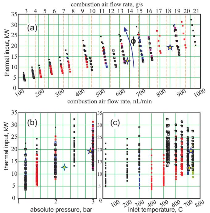
**Figure 5: Burner thermal input versus: a) combustion air flow rate ( $\omega$ ); b) pressure ( $p$ ); and c) inlet temperature ( $T_{in}$ ). Relation between  $\omega$ ,  $p$ ,  $T_{in}$  and  $\phi$  is given in Figure 3. Relation to micro turbine operating points: ★ - base load; ✦ - 50% load.**
