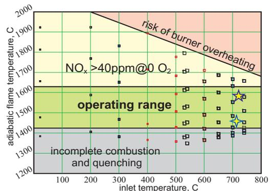
**Figure 8: Experimental points on the plane of adiabatic flame temperature – inlet temperature. Relation between  $\omega$ ,  $p$ ,  $T_{in}$  and  $\phi$  is given in Figure 3. Relation to micro turbine operating points: ★ - base load; ◆ - 50% load.**
