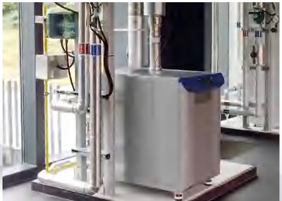
HySa, South Africa: performance of hydrogen combustion in various H 2 /CH 4 /CO 2 mixes
